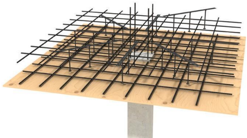
'Top down' installation. Rail is tied to the main reinforcement
