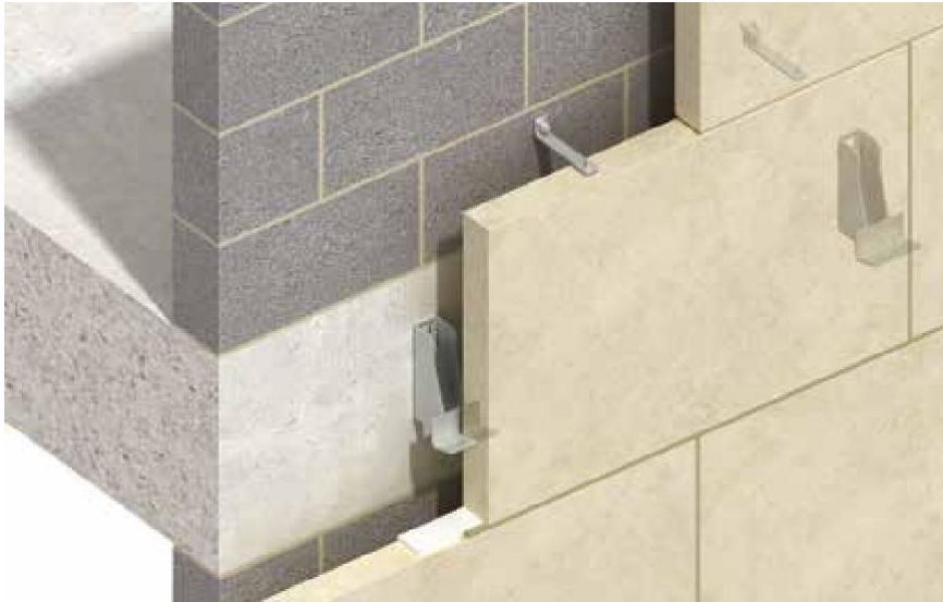
MDA System Supporting Brickwork Curved on Plan
