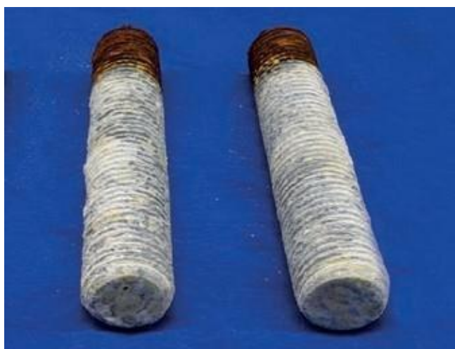
HMR rod end thread after salt spray test for 480 h.
