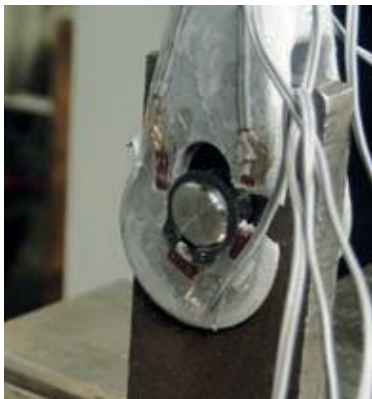
Traction tests on an M16 fork with a breaking load of 150 kN. Fig. TU Munique
